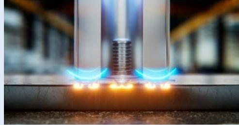
Ultrasonic energy is applied. Within a second the localized thermoplastic melting generates a strong form-locking.
